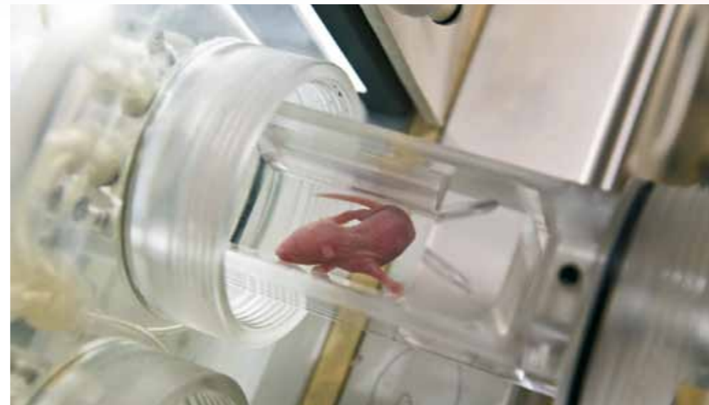
Figure 3: Flow-through plethysmograph with electrodes embedded in the floor
